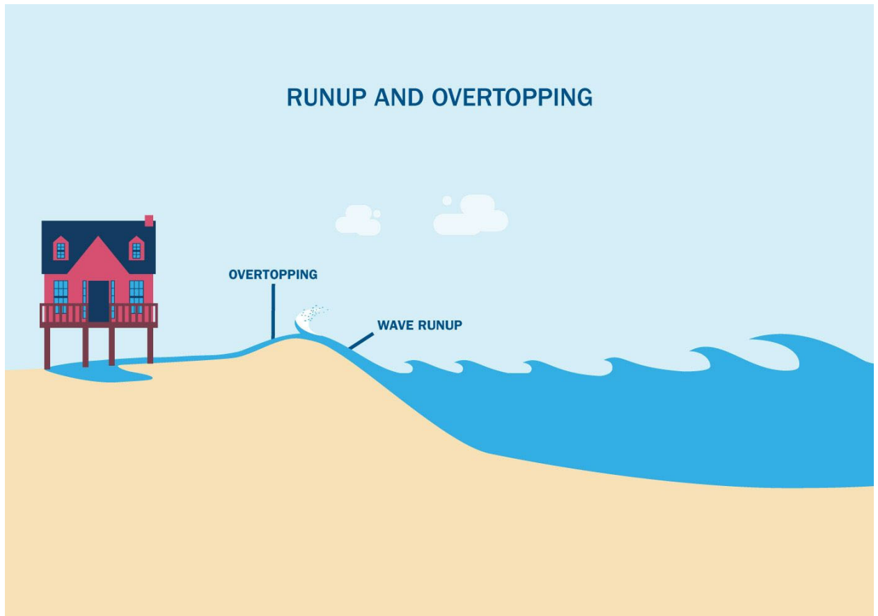
Figure 5b: Wave Overtopping Schematic
